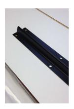
b) ALIGN STIFFENER TO BE 3" FROM LONG EDGES OF TOP – ALIGN CENTERED LENGTHWISE
