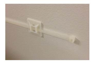
d) FEED TIE THROUGH HOLDER ON UNIT BACK – FEED THROUGH CONNECTOR
