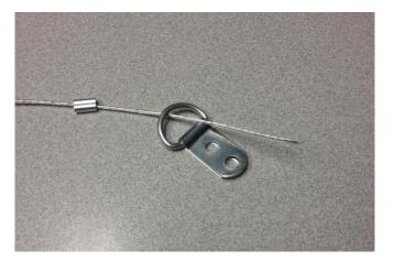
d) BEND BACK WIRE AT MIRROR HANGING LOOP & TWIST WIRE TIGHTLY NO LESS THAN FOUR TIMES
