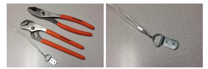
g) DUPLICATE ON OPPOSITE SIDE OF WIRE – ATTACH MIRROR HANGER LOOPS TO BACK OF MIRROR FRAME WITH SELF TAPPING SCREWS PROVIDED
