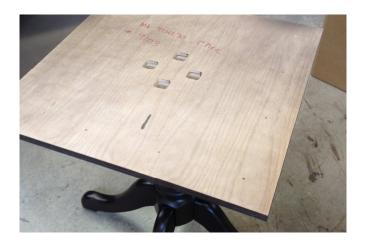
d) USING HARDWARE PROVIDED (Qty 4: 5/16-18 Hex Nut & Qty 4: 5/16 Flat Washer) – ATTACH BATTEN TO BASE (requires 1/2" deep well socket)
