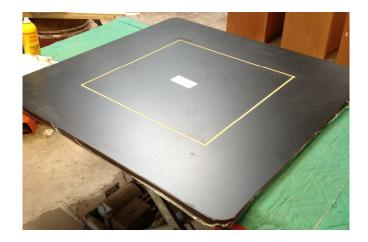
f) FLIP PEDESTAL ASSEMBLY AND ALIGN WITH GROOVE & PILOT HOLES ON BOTTOM OF TOP
